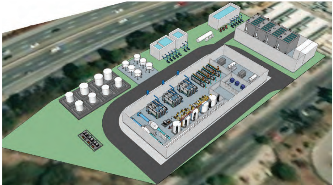
Figure 8.12 Isometric View of DPR Treatment Train in Santa Barbara
